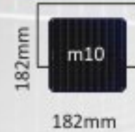
M10 PERC MONOKRİSTAL SOLAR HÜCRE
